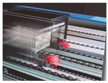
*Fig. 4: This device (tilting sensor) was developed especially for eKanban applications*
